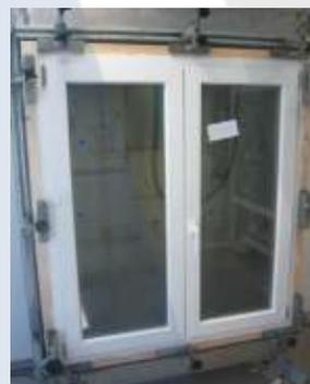
**Permeabilidad al aire****Muestra cerrada****CLASE 4****Muestra en posición de microventilación****CLASE 1**
